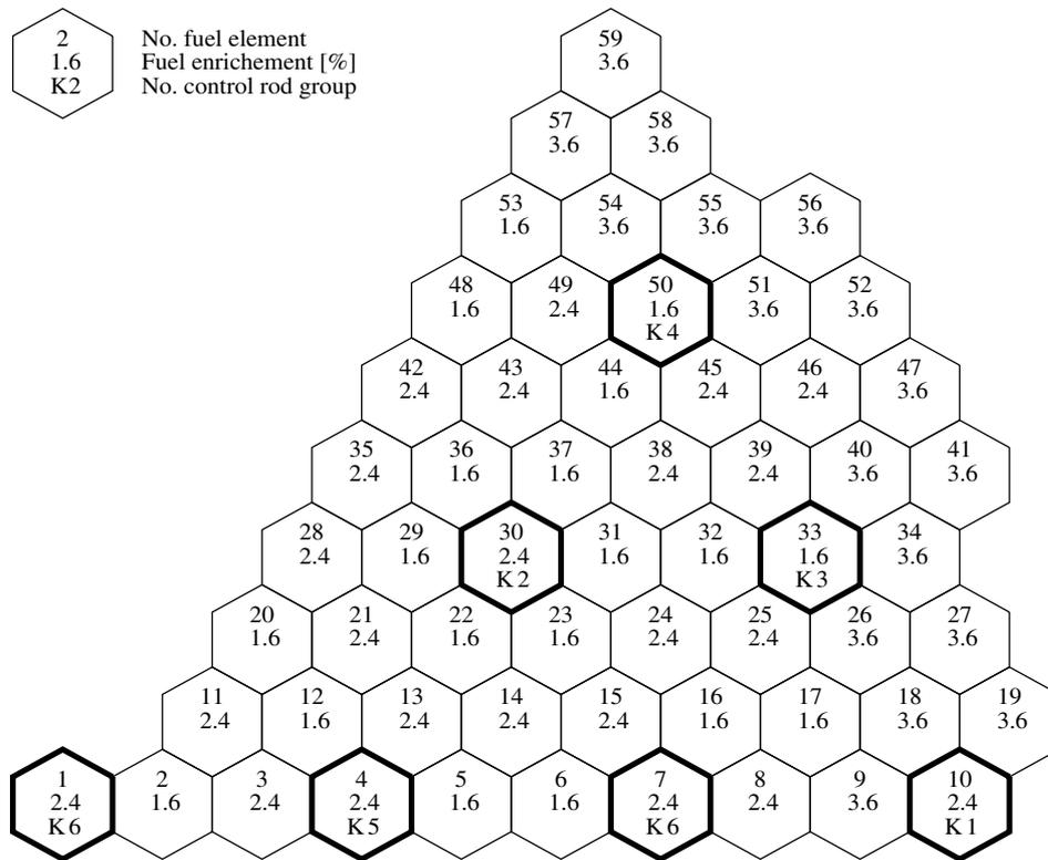
Fig. 1 Horizontal map of the VVER-440 reactor core in 60° core symmetry for this benchmark.
