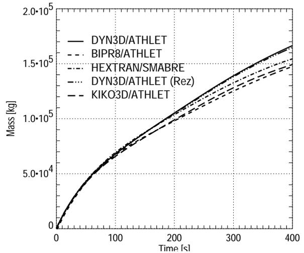
Fig. 4 Integrated leak mass
