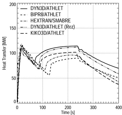
Fig. 11 Averaged heat transfer in the SG of the loops without pressurizer
