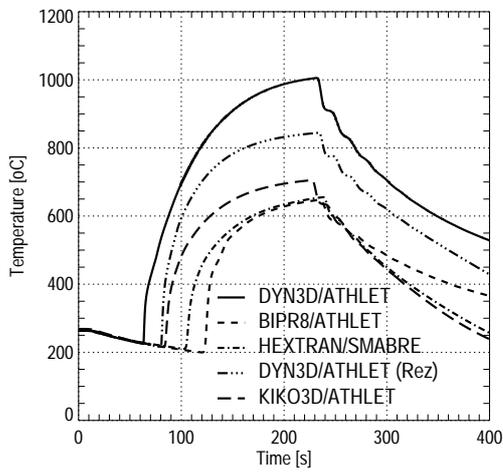
Fig. 9 Maximum fuel centerline temperature
