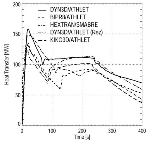
Fig. 10 Heat transfer in the SG of the loop with the pressurizer
