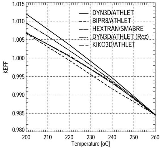
Fig. 2 Keff of stationary calculations with different inlet temperatures
